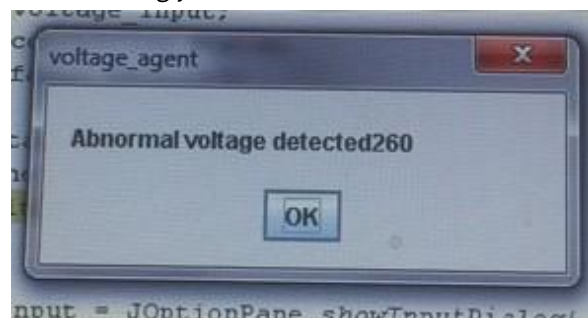
Figure 7: Switch (Voltage) Agent detecting and reporting abnormal voltage
